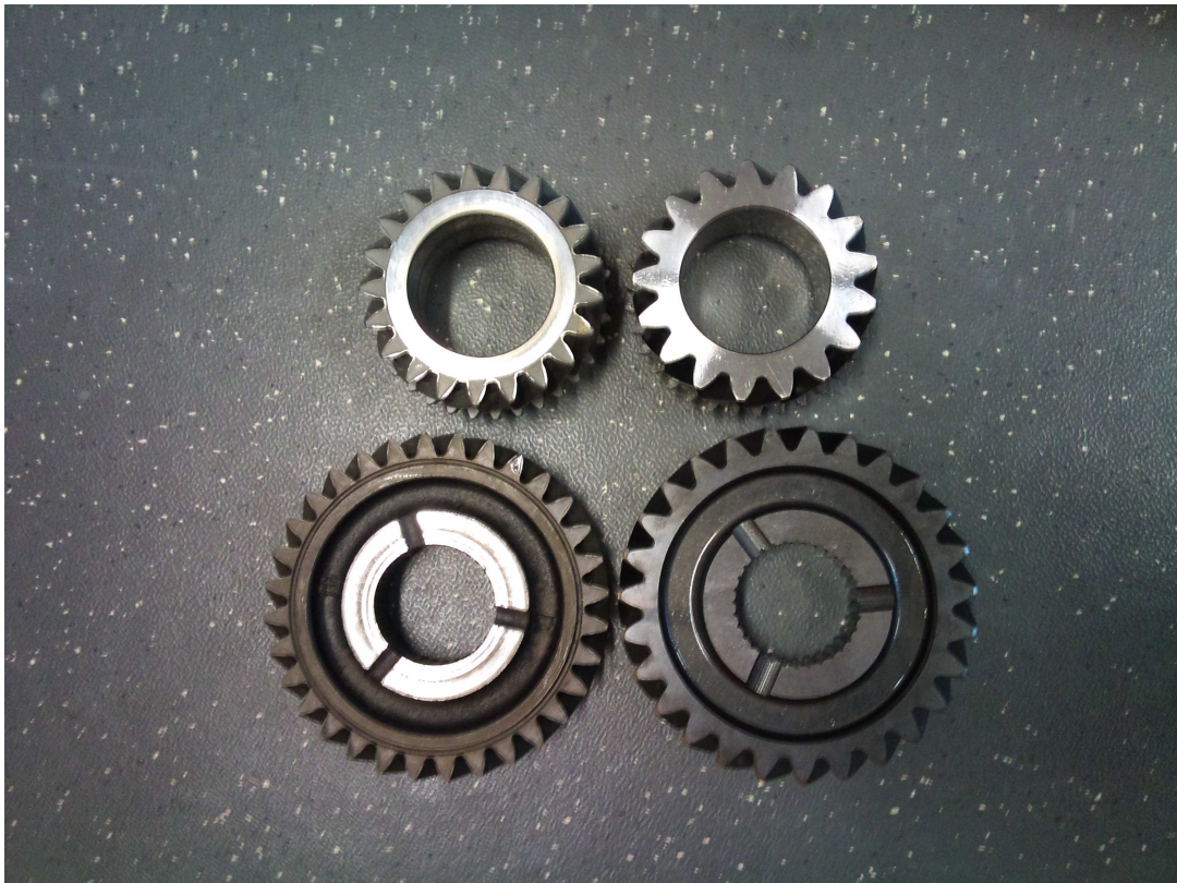
Difference 3 rd gear old (left) to 3 rd gear new (right): 5mm tooth base vs. 7mm tooth base
